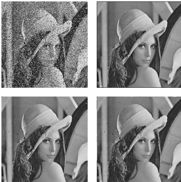
Fig. 2. The Lena image with 20% impulse noise, and the results of FIDRM (top right), EMF (lower left) and classical median filter (lower right)
