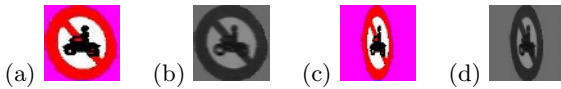
Fig. 9. Four version of images used for road sign recognition. (a) Normalized color image, (b) normalized gray image, (c) non-normalized color image, and (d) non-normalized gray image.
