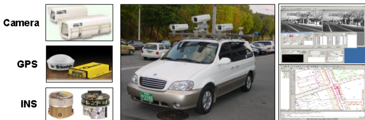
Fig. 1. 4S-Van: a mobile mapping system
