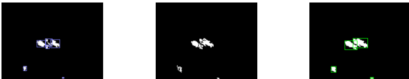
(a) Thresholded image difference (b) Morphological processed edges (c) Superimposition of a) and b)
