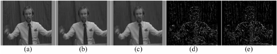
Fig. 4. Trevor frame #131. (a): Original frame, (b): reconstructed with full analysis of modes, (c): reconstructed with proposed scheme, (d): Difference image with full analysis, (e): Difference image with proposed scheme.
