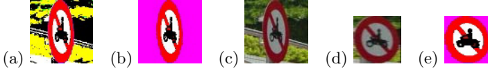
Fig. 4. Preprocessing and normalization. (a) Detected road sign ( 56 \times 127 pixels), (b) detected road sign with background masked off, (c) extracted road signs, (d) normalized road sign ( 96 \times 96 pixels), and (e) scene image for recognition.
