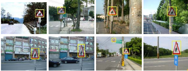
Fig. 6. Road sign in the variations of scale and skew. Detected road signs are marked by rectangles.
