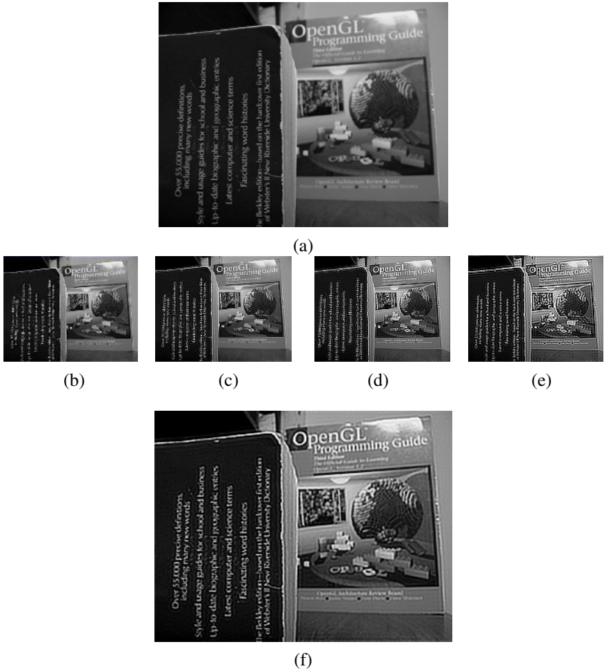
Fig. 2. Experimental results: (a) The source image, (b)-(e) restored image using a priori set of PSFs, and (f) the restored image based on image fusion
