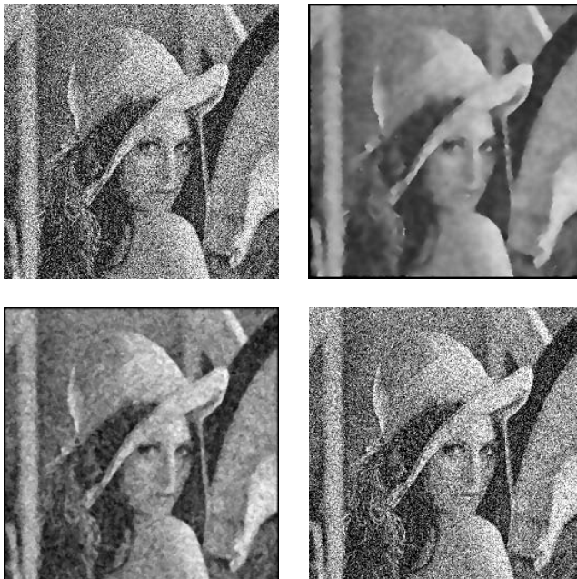
Fig. 3. The Lena image with \sigma = 50 (gaussian noise), and the results of GOA (top right), IFCF (lower left), and classical gaussian filter (lower right)
