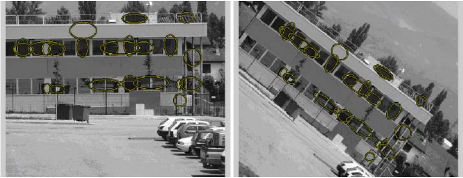
Fig. 6. Some of the repeated regions in two images taken in different zooming position and rotational angle
